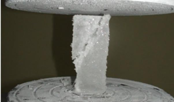
Fig. 5 Compressive strength test of model ice
